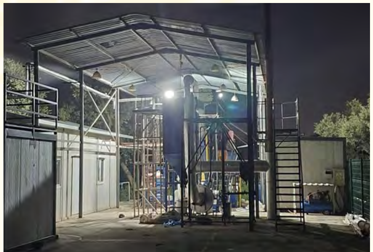
40 kW thermal capacity fluidized bed unit
